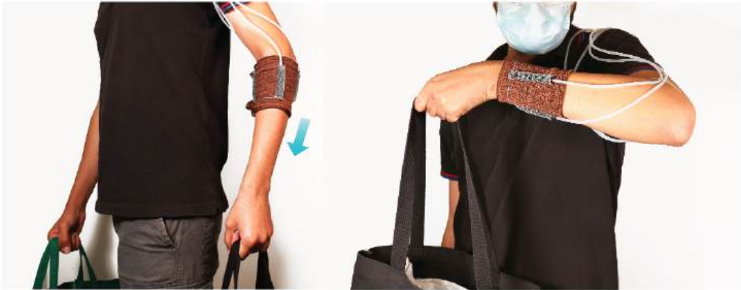
Figure 30: KnitSkin, as a wearable interface carrying a microphone, relocates to a suitable location on the arm when answering a phone call.
