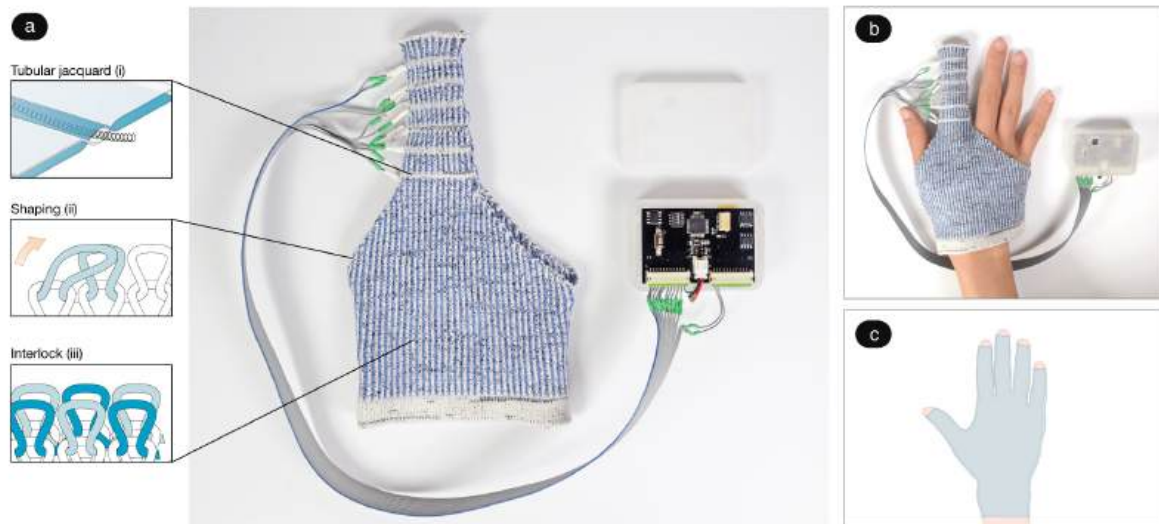
Figure 35: (a) KnitDema system in which the finger sleeve is knit with a combination of (i) tubular jacquard, (ii) shaping, and (iii) interlock structure. The tubular structure creates "channels" to incorporate SMA springs. The substrate also uses a shaping structure to conform the substrate to the rest of the fingers. (b) KnitDema finger sleeve device worn on a hand. (c) Future implementation of a full-hand KnitDema device.
