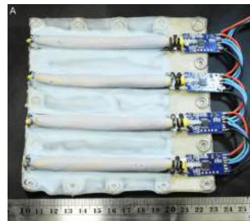
(b) Pneumatic actuators in OmniSkin [26] are glued onto fabric.
