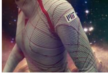
Figure 3: The BioSuit, embedded with shape memory alloy, is designed as an alternative to the existing stiff and gas-filled space suits.
