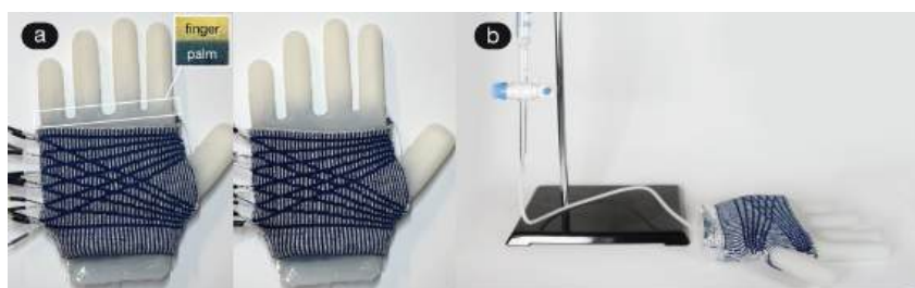
Figure 52: (a) Experimental setup to observe backflow displacement of fluid from the fingers to the hand. The sponges utilized exhibited uniform porosity. The image on the right shows no discernible displacement of pigment from the onset (left). (b) Setup to characterize compression bands in the palm. The silicone mock hand was positioned flat embedded with 12 SMA compression bands.
