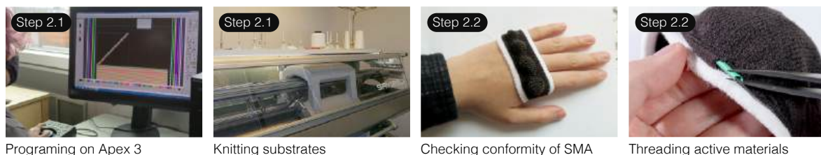
Figure 14: Step 2. Fabrication process of KnitDermis. Designs of KnitDermis substrates are digitally programmed on Apex 3. Once knitted with desired yarns and appropriate stitch cam setting, substrates are placed on body to see if they conform to underlying body geometry and the SMA is placed fittingly. Prior to threading active materials, soft and pliant tubes are inserted first to protect substrates.
