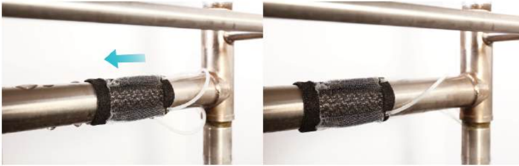
Figure 31: The KnitSkin ground layer can be knitted with a wide range of materials, including water soluble PVA yarn. When KnitSkin travels along a pipe and becomes exposed to a leakage point, the PVA yarn dissolves, forming a protective layer on the point of leakage.
