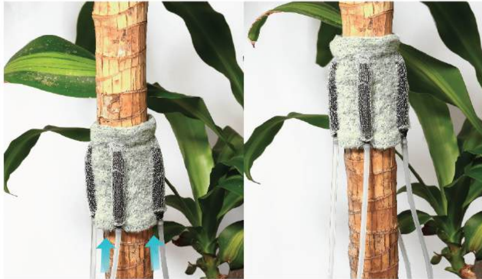
Figure 32: By modifying channels into pockets for a portable pesticide dispenser, KnitSkin can further work as an agricultural robot.
