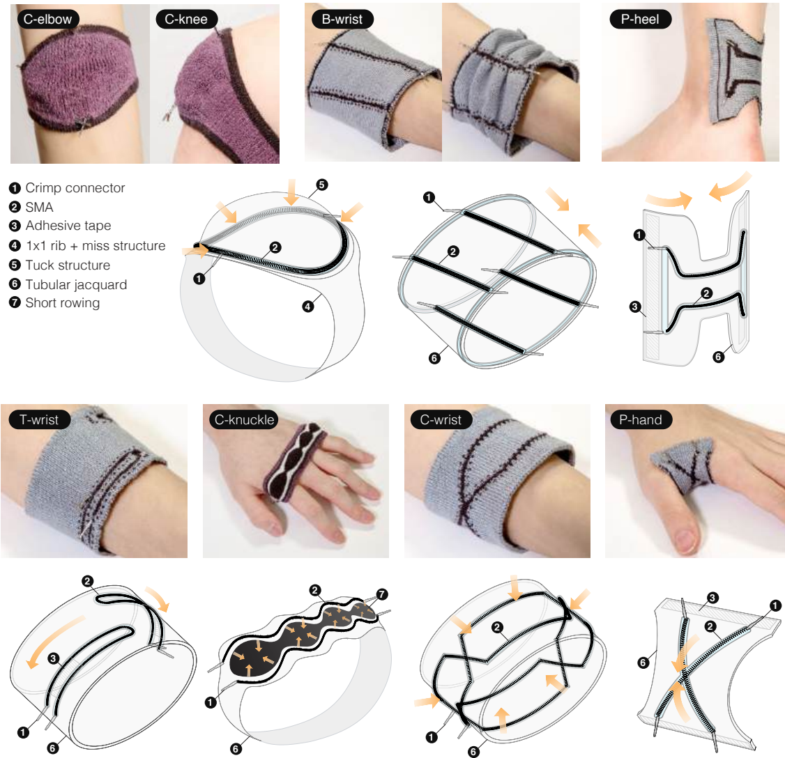
Figure 15: Summary of eight KnitDermis case studies. Depending on haptic feedback of interest, each case study variously configures design factors to conform to specific body locations. B-wrist and C-wrist adopt self-shifting mechanism whereas the remainder utilizes skin-shifting mechanism.
