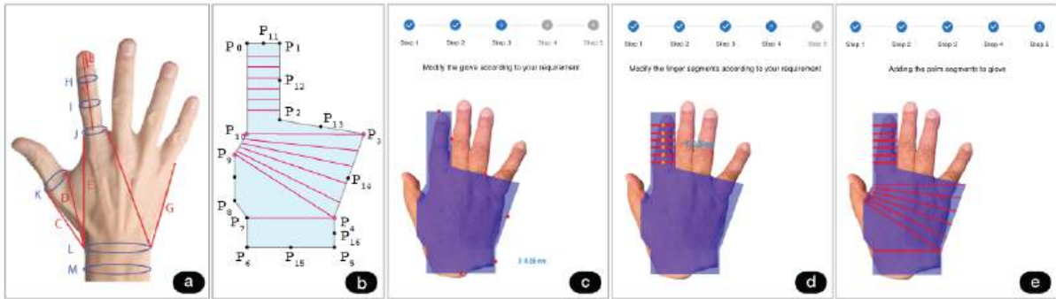
Figure 53: MediKnit design tool provides: (a) Visual guidance for thirteen hand measurements for customization; (b) Backend algorithm converts the measurements to 18 coordinate points; (c) and (d) A glove template is generated based on these coordinates, with options for therapists to adjust both the template and SMA channels; (e) The design tool then creates a machine-readable file.
